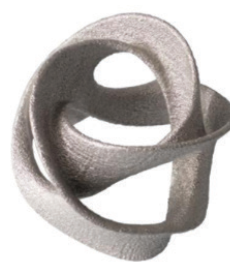
Figure 7. Inkjet 3D printed complex metal part. Source: https://www.materialsampleshop.com/products/metal-3d-printing-inkjet-route
