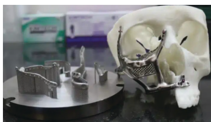
Figure 1. Human face implant (Ti- laser PBF).
