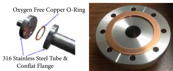
Figure 5: Placement of copper gaskets on the flanges to make the sealing
